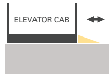
Slab with RAM's No Pit (small ramp required for 2in rise)
